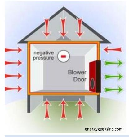
A Blower Door Test induces a pressure difference between inside and outside
