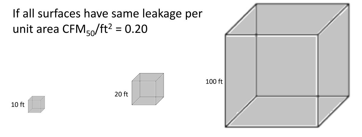
$CFM_{50}/ft^2 = 0.20$ ACH50 = 600\*0.20/1000\*60 = 7.2  $CFM_{50}/ft^2 = 0.20$ ACH50 = 2400\*0.20/8000\*60 = 3.6 CFM<sub>50</sub>/ft<sup>2</sup> = 0.20 ACH50 = 60000\*0.20/1000000\*60 = 0.72
